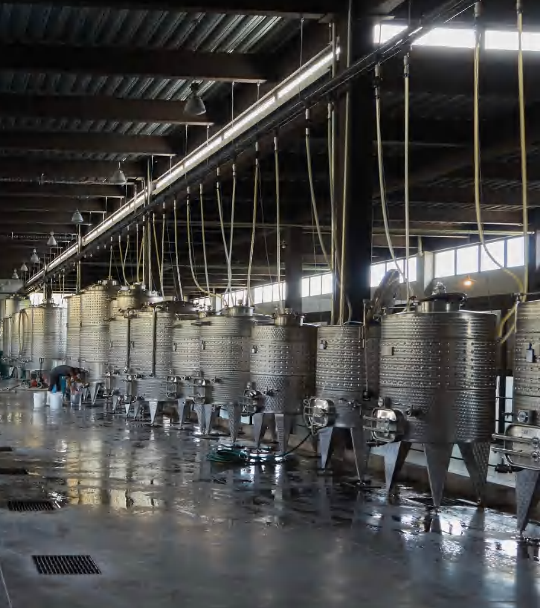
Stainless steel tanks for the most fermentation, at Viñedo San Miguel.
